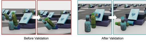
Fig. 6. Dominoes solutions. Left: A high-risk strategy that places the green bottle on the can to tip it toward the target; it occasionally succeeds but is sensitive to placement noise. Right: The selected robust strategy, which places the bottle between the objects and rolls the can down the ramp. Validation favors the solution with higher expected reward.
